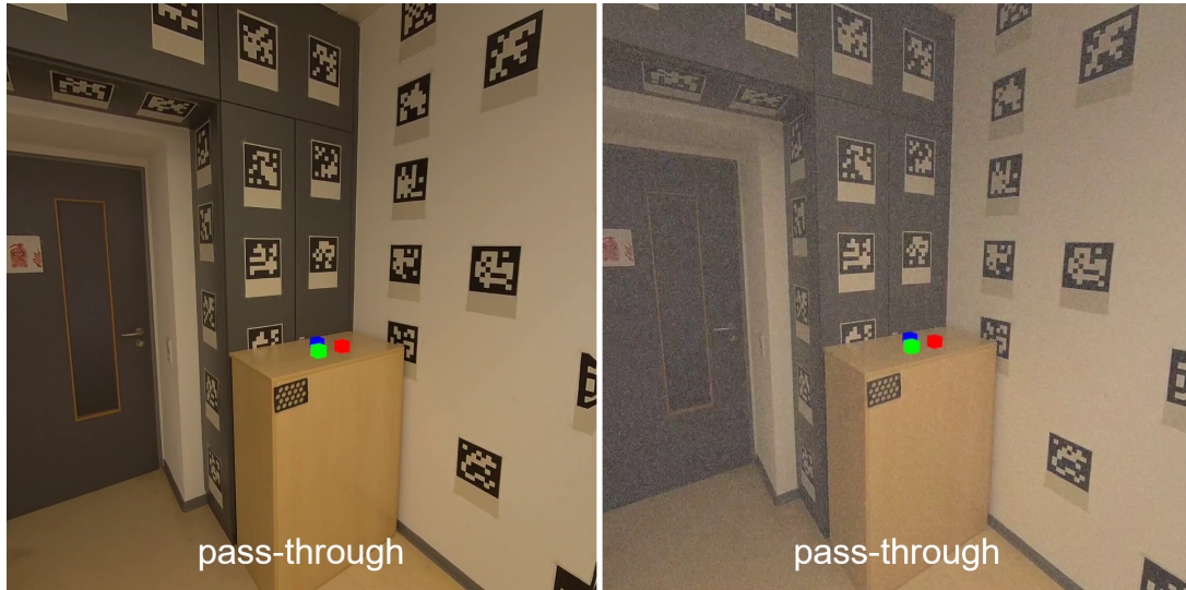
Figure 4.3: Effect of the visual noise on the pass-through video feed
