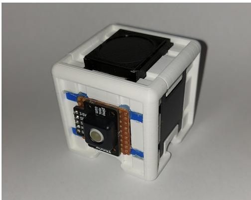
(c) The second controller. Visible here: trackball (on the side) and touchpad (on the top)
