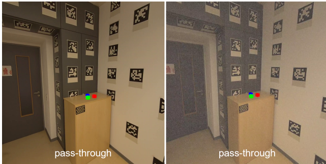
Figure 4: Effect of the visual noise on the pass-through video feed
